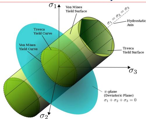
The von Mises yield surfaces in principal stress coordinates circumscribes a cylinder with radius  $\sqrt{3}\sigma_y$  around the hydrostatic axis. Also shown is Tresca's hexagonal yield surface. Picture from [http://en.wikipedia.org/wiki/Von\\_Mises\\_yield\\_criterion](http://en.wikipedia.org/wiki/Von_Mises_yield_criterion)
